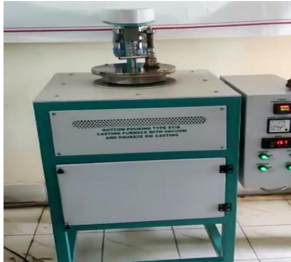
Pouring Type Stir casting furnace with Vacuum and Squeeze Die Casting”
